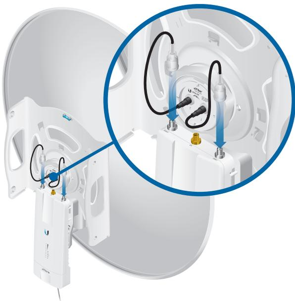
3. Attach the *External GPS Antenna* to the RF connector labeled *GPS*. Then, place the magnetic *External GPS Antenna* on the bracket (this is temporary; you will mount the *External GPS Antenna* on the *GPS Antenna Mount* at the site).
