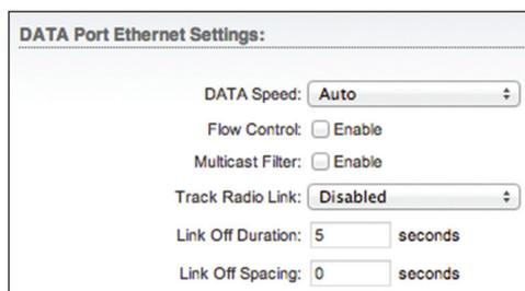
**DATA Speed** This is the speed of the *Data* port. By default, the option is **Auto**. The AF-5X automatically negotiates transmission parameters, such as speed and duplex, with its counterpart. In this process, the networked devices first share their capabilities and then choose the fastest transmission mode they both support.
