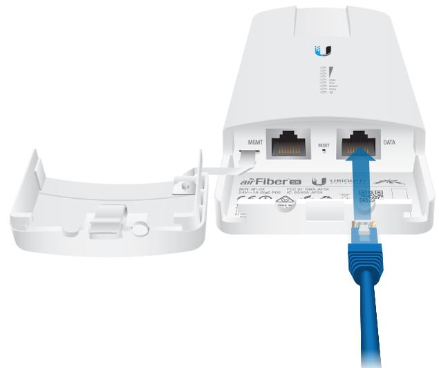
3. Connect the Ethernet cable from the *DATA* port to the Ethernet port labeled **POE** on the *airFiber PoE Adapter*.
