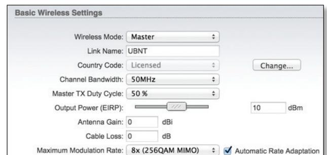
**Wireless Mode** By default, the Wireless Mode is *Slave*. You must configure one AF-5X as **Master** because each PtP link must have one *Master*.
