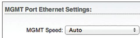
**MGMT Speed** This is the speed of the *Management* port. By default, the option is **Auto**. The AF-5X automatically negotiates transmission parameters, such as speed and duplex, with its counterpart. In this process, the networked devices first share their capabilities and then choose the fastest transmission mode they both support.
