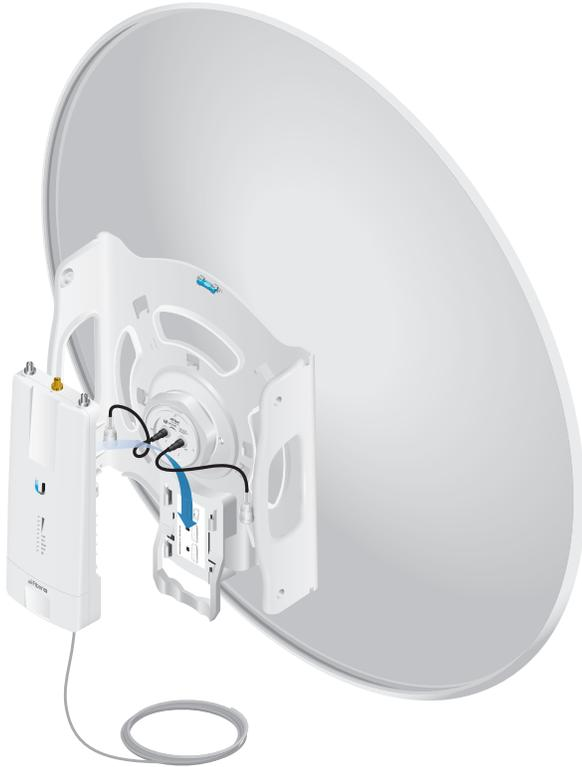
2. Attach the RF cables from the antenna feed to the RF connectors on the AF-5X in this combination: +45° to Chain 0 and -45° to Chain 1.
