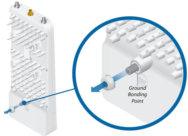
2. Attach a ground wire (min. 10 AWG or 5 mm<sup>2</sup>) to the lug and replace the nut to secure the wire.
