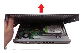
Step3 With your hand supporting the HDD when turn unit upside down, remove 4 screws from the bottom of case.
